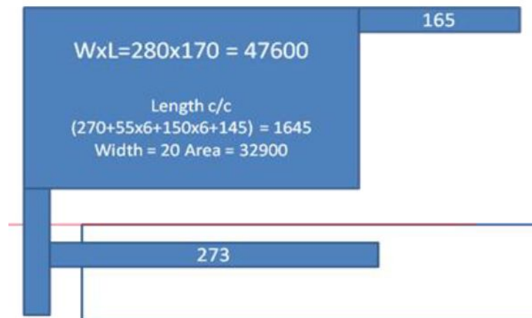
Figure 1 Required patch area and layout
