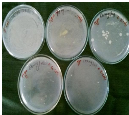
Figure 3: Effect of MgO nanoparticle on water sample plate 1 ( MgO + E.coli ) shows no growth & Plate 2 ( without MgO + E.coli )cultivated in NA media shows Mat growth
