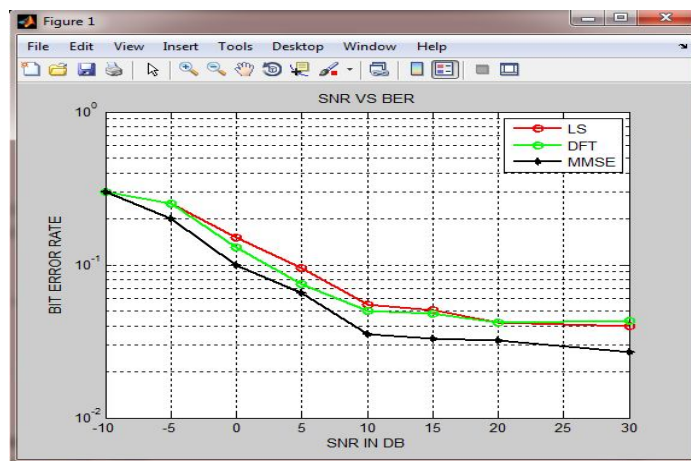
Figure 5: Graph between BER vs. SNR for LS, MMSE and DFT channel estimators
