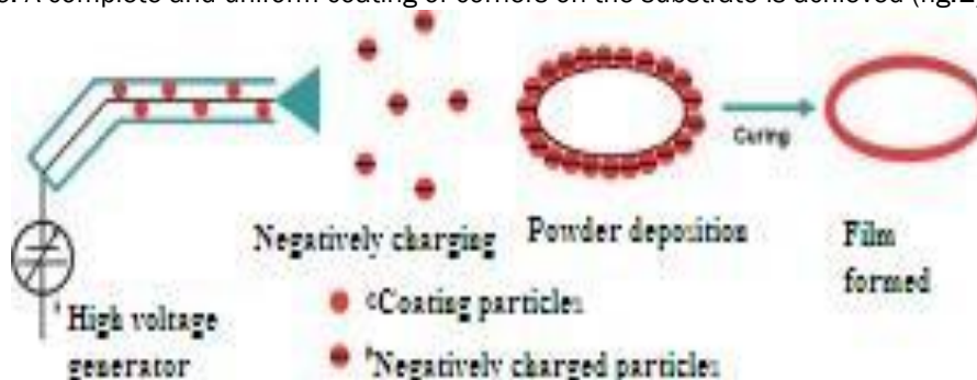
Figure1: Mechanism of electrostatic coating [6].
