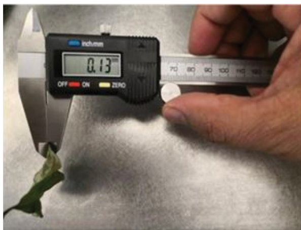
Figure 4. Demonstration of measuring the thickness of leaf using Vernier calliper.
