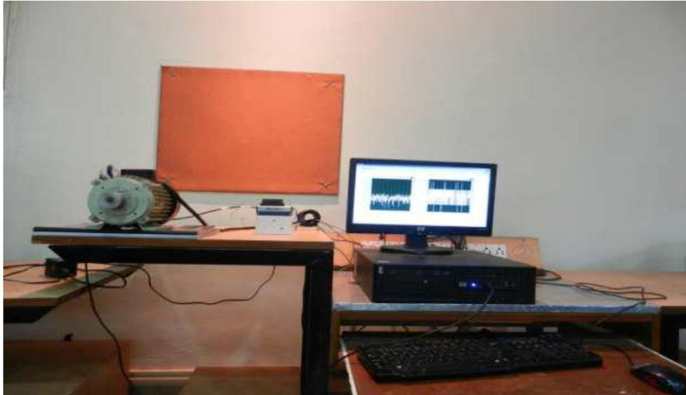
Fig. 2 Test bench for current condition monitoring
