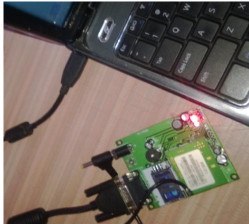
Fig.6 Connection between PC and GSM SIM 300 using RS-232 cable
