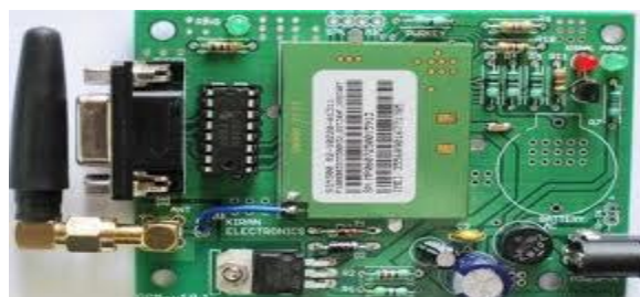
Fig.5 GSM SIM 300 modem
