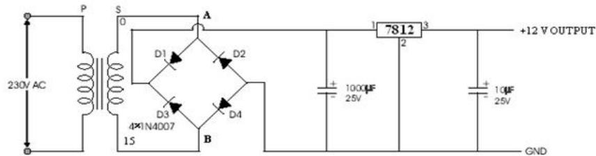
Fig.6 Circuit diagram for power supply
