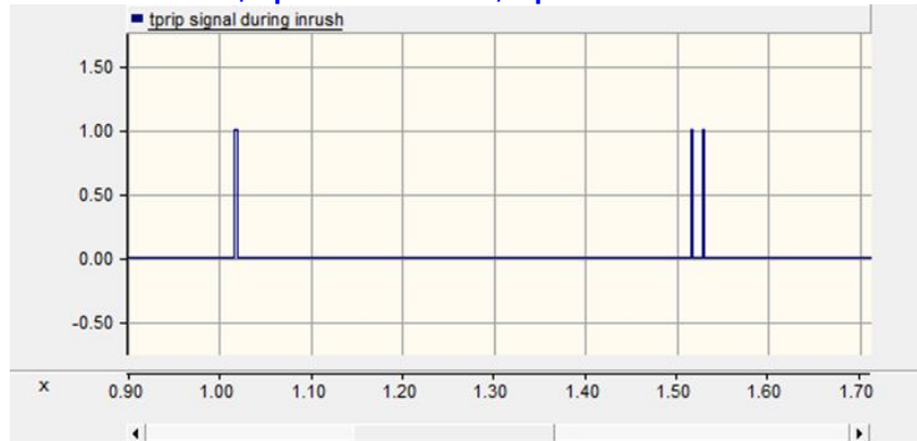
Fig. 12. Mal-operation of relay due to inrush current
