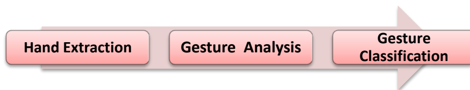
Fig.2. Recognition gesture system stages.
