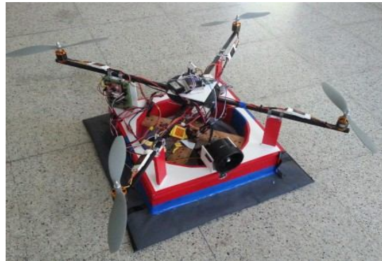
Fig.2. Implementation of prototype of the quadrotor hovercraft
