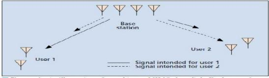
Figure 1. An illustration of a multi-user MIMO downlink. Each user often receives data intended for other users.
