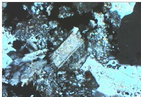
Fig. 2 - Image of sandstone in the polarizing microscope in transmission light with lens 20 x , with analyzer
