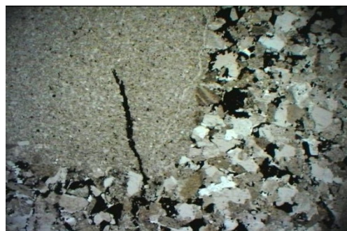
Fig. 3 – Image of aleurolite including in sandstone in the polarizing microscope in transmission light with lens 2,5 x , without analyzer
