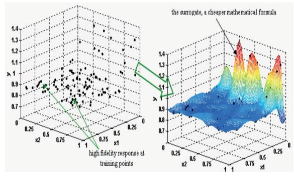
Figure 1: A sample surrogate model for two variables constructed based on simulation data set.
