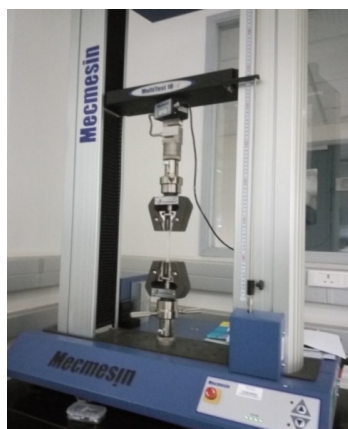
Figure 5. Computerized UTM apparatus for tensile.
