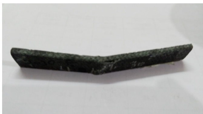
Figure 9. Flexural tested specimen.
