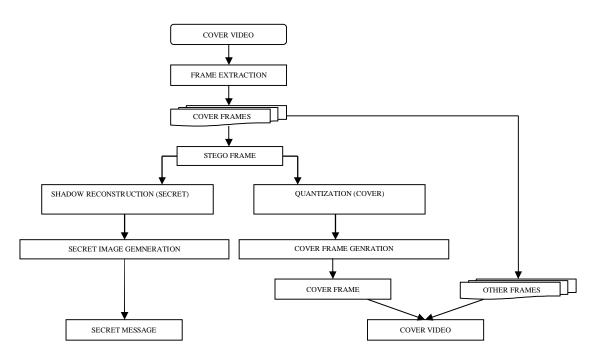
Fig.3 Block Diagram (Decryption System)
