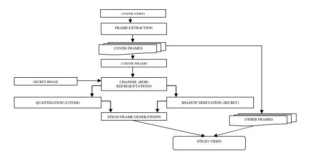
Fig.2 Block Diagram (Encryption System)
