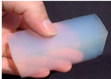
Fig.1 Aero gel: evacuated Nano pores in SiO 2 matrix
