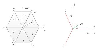
Fig 8 (a) Space Vector Diagram for 2 Phase Inverter,(b) Diagram of Reference Vector in abc and  $\alpha\beta$  axis
