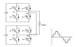
Fig1. Five level cascaded H-bridge inverter
