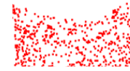
Fig. (3b): After reduction, it has 753 points and is fitted to plane and the error is 0.0087.
