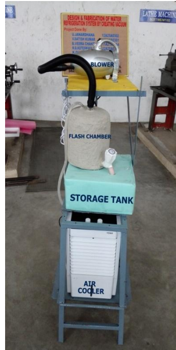
Fig.7 Fabricated model of water refrigeration system by creating vacuum
