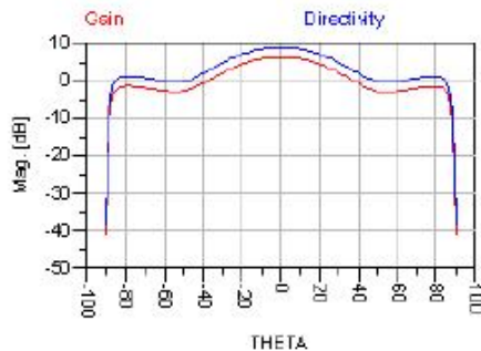
Fig.11 Gain and Directivity of Proposed Microstrip antenna
