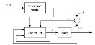
Fig. 9 General structure to control a plant with reference model
