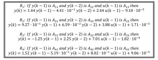
Fig. 5 Second TS model of the conical tank of [31]
