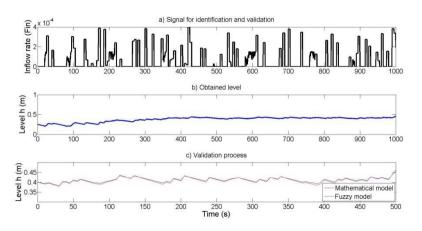
Fig. 4 Signals for identification and validation
