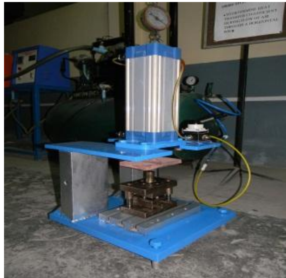
Fig. 1 Experimental Setup of Pneumatic Punch
