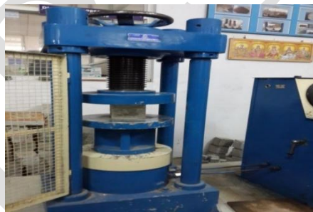
Fig. 6 Compression test for cube
