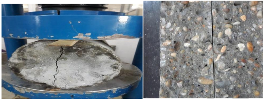
Fig. 7 split tensile test for cylinder
