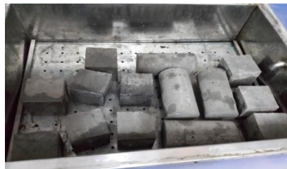
Fig. 5 Steam curing tank
