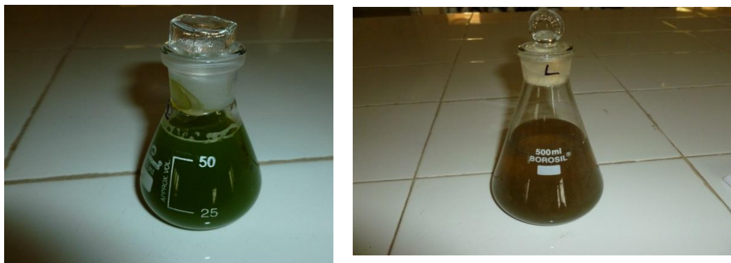
Figure 1. Color change of A. sessilis plant leaf extract containing silver before (left) and after (right) synthesis of silver nanoparticles.
