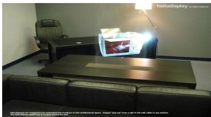
Fig. 2 [7] Heliodisplay projecting image into free space
