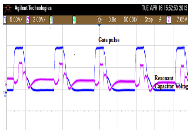
Fig 11 Soft Switching phenomenon observed on DSO
