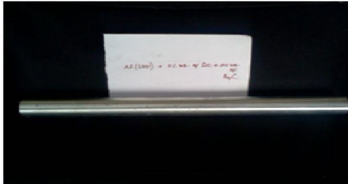
Figure 4.1 Al (6351) + 5 wt. % of SiC + 5 wt. % of B 4 C
