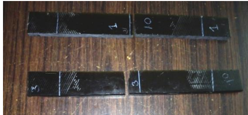
Fig. 1 Composite with 0% fiber prepared using Hand layup procedure
