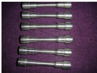
Fig.2.9: Tension test specimens
