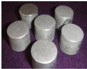
Fig.2.7: Hardness test specimens
