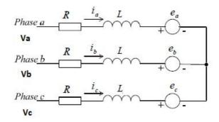
Fig 1:Electrical equivalent circuit of BLDC motor
