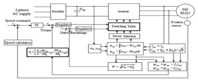
Fig 2:Block diagram of direct torque control of BLDC motor
