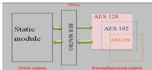
Fig. 7 Block Diagram of AES Algorithm with PR
