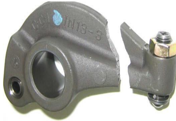
Fig.8. Fracture at the neck of the rocker arm
