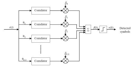
Fig.1 Conventional rake receiver
