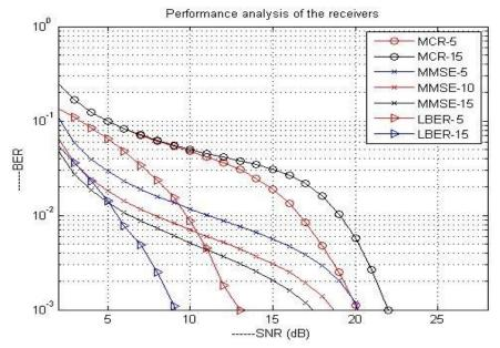
Fig.2Performance analysis of the receivers
