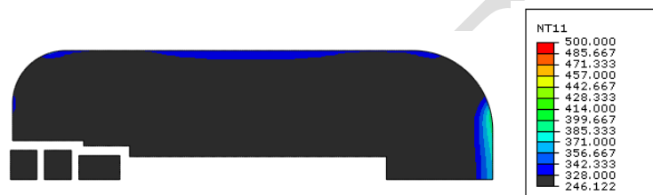
Fig. 15. Temperature Profile in Molten Lead after 2 Minutes into Post Fire
