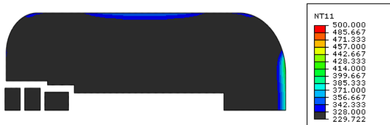
Fig. 11. Temperature Distribution in Molten Lead after 30 Minute in Fire
