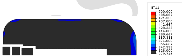
Fig. 16. Temperature Profile in Molten Lead after 7 Minutes into Post Fire
